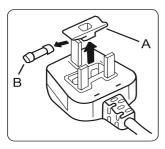
The mains lead of this appliance has been fitted with a BS 1363A 13A fused plug. To change a fuse in this type of plug, follow the steps below:
